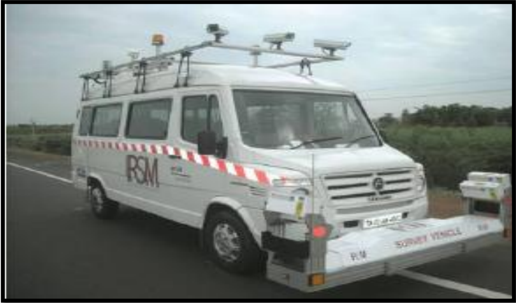
Photo 15: Network Survey Vehicle Collecting data on RBI Grade81 Stretch
