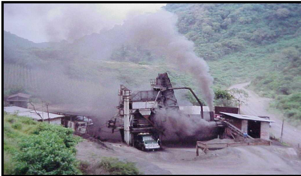
Photo 3: Pollution during Hot Mixing of Bitumen
