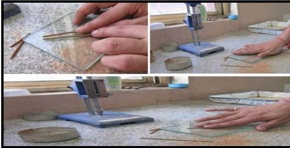
Photo 2.4: Plastic Limit Test in Progress
