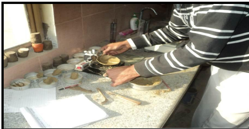
Photo 2.2: Liquid Limit in Progress by Mechanical Method
