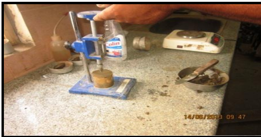
Photo 2.3: Liquid Limit Test in Progress by Cone Penetrometer Apparatus
