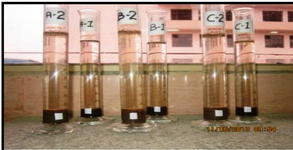
Photo 2.5: Free Swell Index Test in Progress
