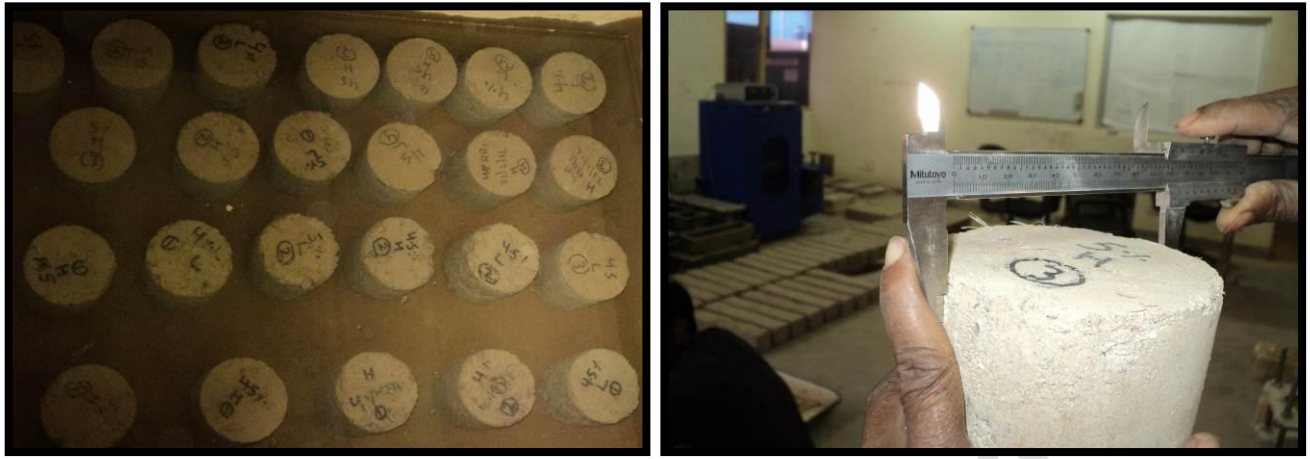
Photo 2.11& 2.12: Durability Test in Progress (Wetting and Drying)
