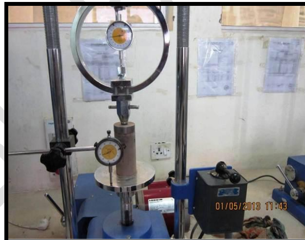
Photo 2.8 & 2.9: UCS test in Progress (For Fine Grain Soil)
