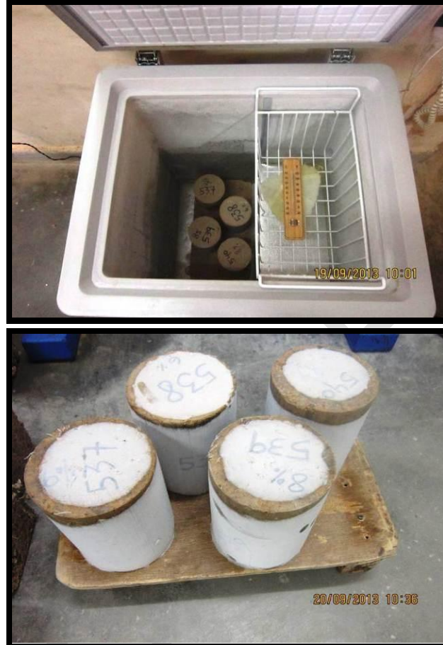
Photo 2.13 & 2.14: Durability Test in Progress (Freezing and Thawing)
