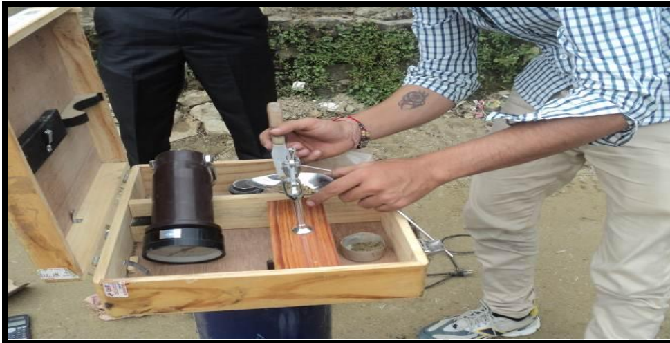
Photo 2.16: Moisture Content Test in Progress
