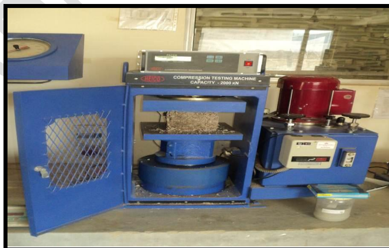
Photo 2.10: UCS Test in Progress (For Coarse Grain Soil)
