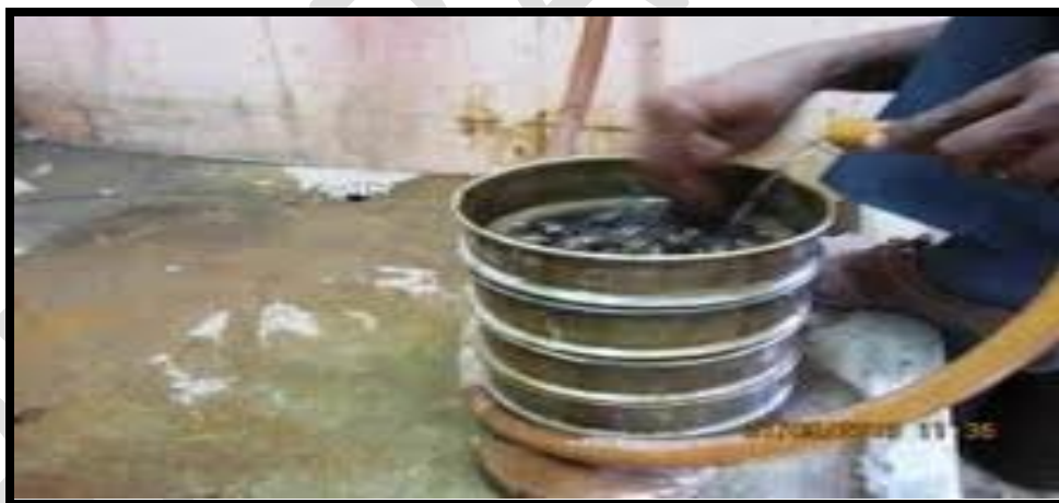
Photo 2.1: Wet Sieving in Progress
