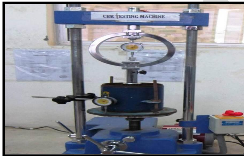
Photo 2.7: CBR Test in Progress
