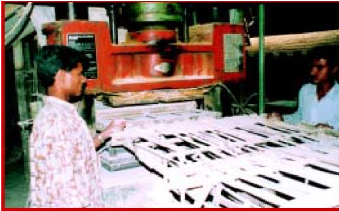
Figure 6.10 : Hydraulic press for pressing tiles
