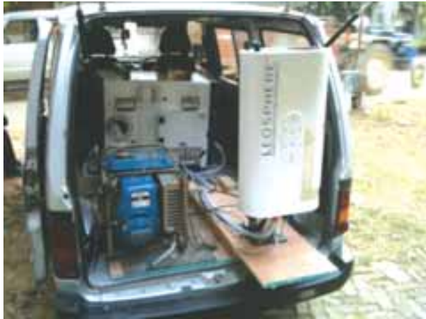
Fig-55. : Lidar based air quality forecasting system
