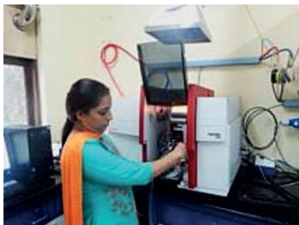
Fig-42. Wood preservative analysis using Atomic Absorption Spectrometer
