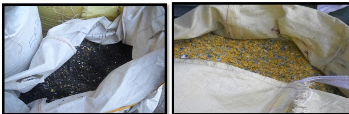
Photo 4: Plastic / Pet bottles graded and shredded into pebbles at a processing plant at Singtam
