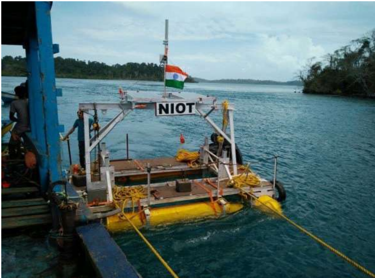
Figure 8: Marine Current Turbine tested at Andaman
