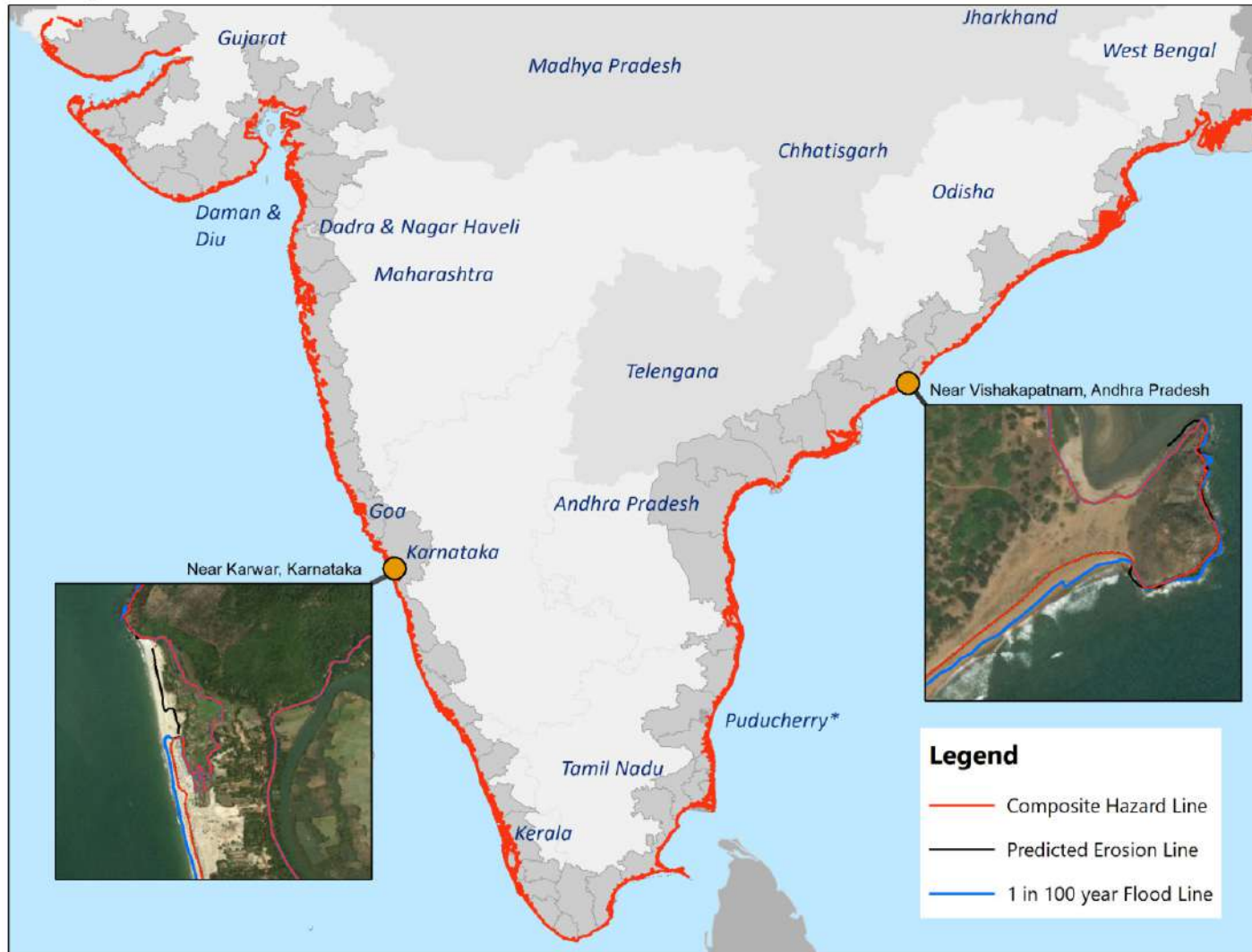
Figure 10: Composite Hazard Line for the coast of India. Insert: West coast: Near Karwar, Karnataka and East Coast: Near Vishakhapatnam, Andhra Pradesh showing 1 in 100 year flood line, 100-year predicted erosion line and composite hazard line
