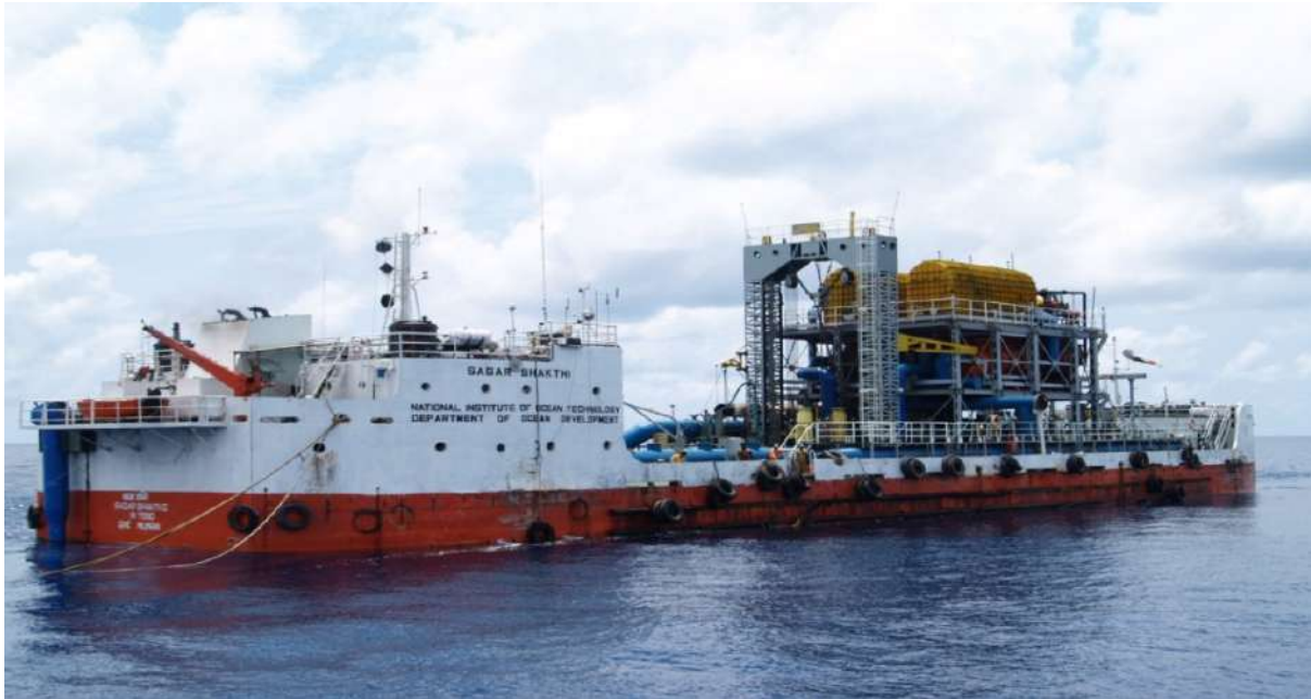
Figure 4: Barge mounted desalination Plant
