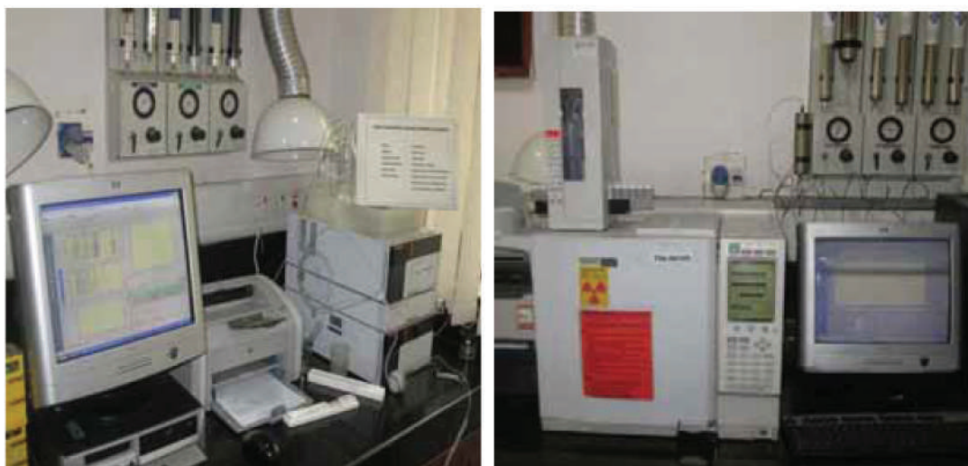
Pesticides Quantification on Gas Chromatographs
