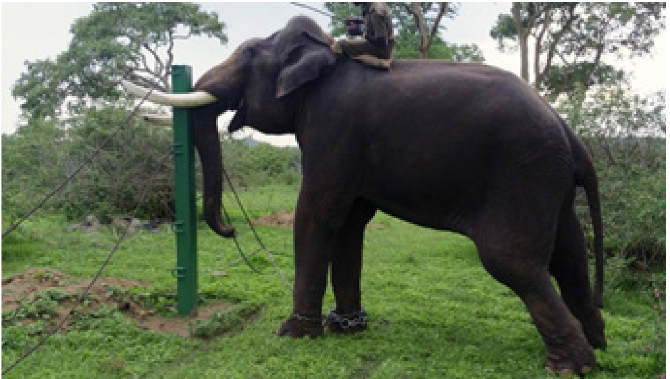
1 - Kumki elephant tests the prototype fence post
