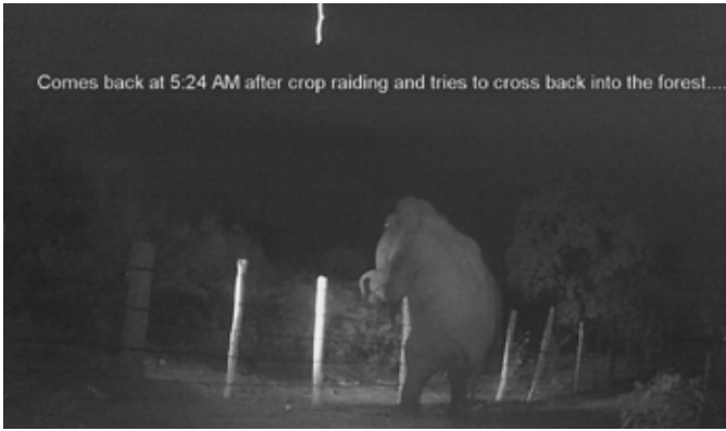
Fig 6 Wild makhna is unable to climb over fence after fixing eucalyptus spacers
