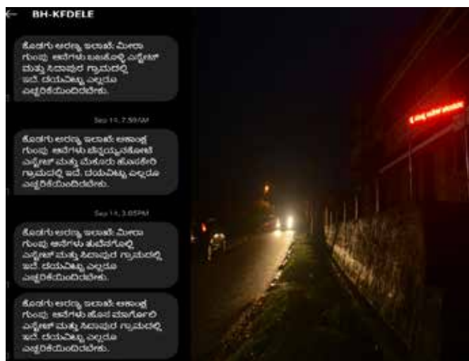
Left: Bulk SMS sent to villagers about location of elephant in Kannada Language Right: Elephant location displayed in GSM enabled LED boards along a village road to alert the motorists and passerby.
